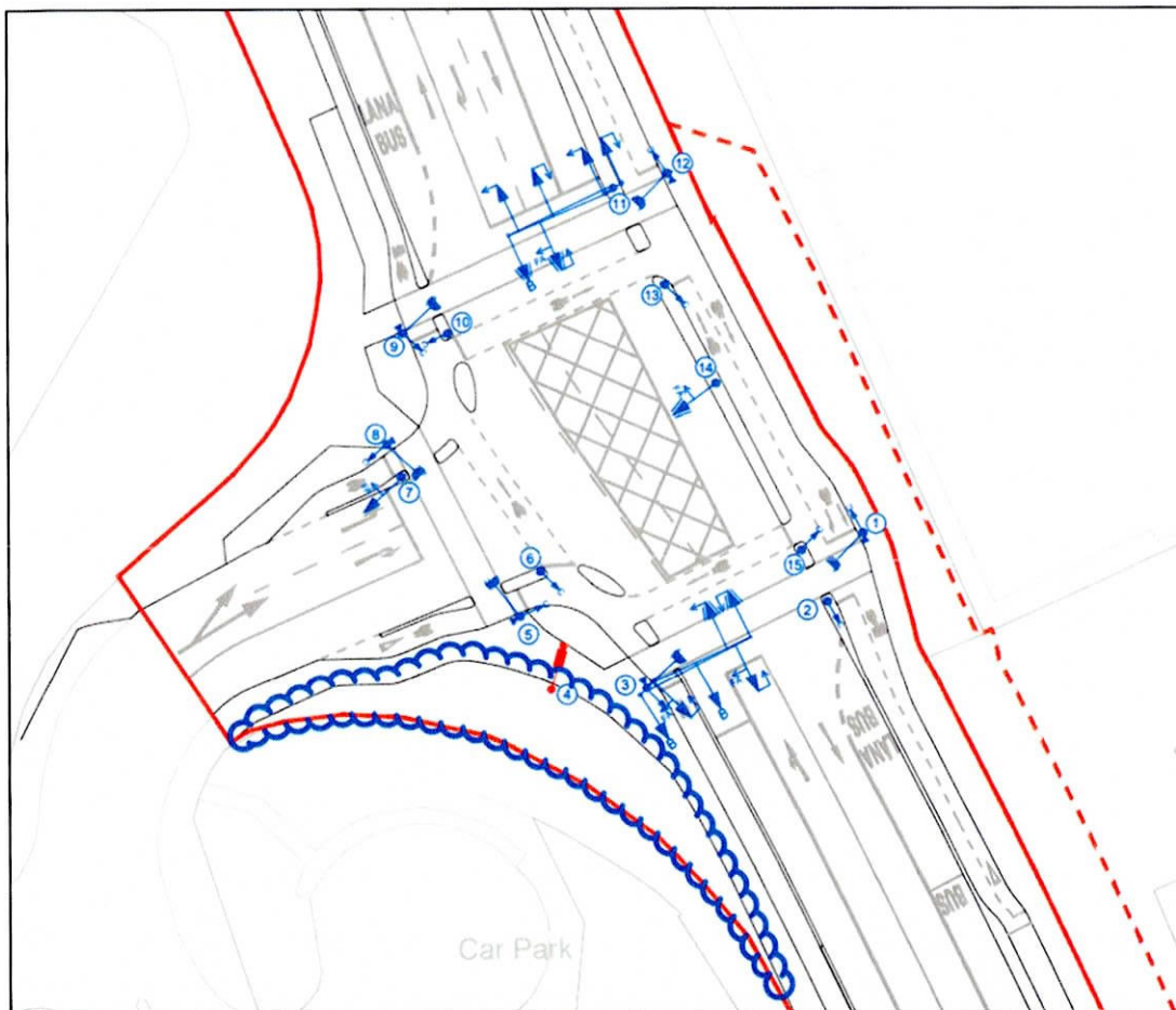
Figure 2: Extract from Proposed Traffic Signal Design Layout (BCIDC-ARP-TSM SJ-1415 XX 00-DR-TR-0012)
